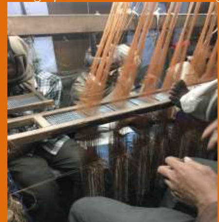
Setting up the loom for sari weaving
